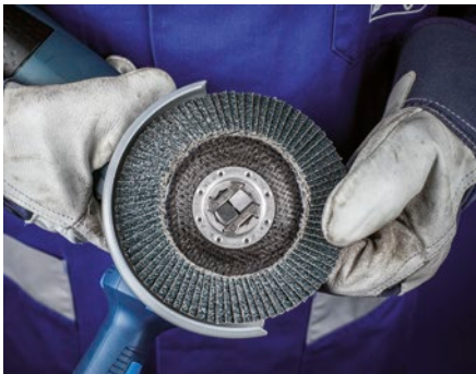
Place the disc on the X-LOCK holder in a form-fitting manner.
