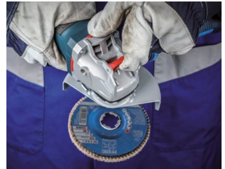
Release the disc by using the lever.
